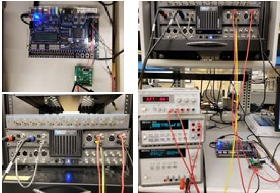
Figure 3.4. Bench test setup for 16-bit R2R linearity measurement
